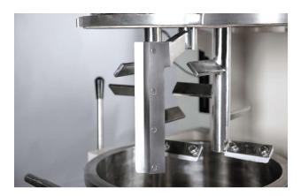
PerMix PDP series Double Planetary Mixer is also called double planetary kneader, because it can be used to handle very viscous materials up to 1,500,000 cPs. Usually PerMix Double Planetary Mixer has two vertically mounted mixing tools which are driven by one gear to move around the central axe of the tank as well as their own axis.
