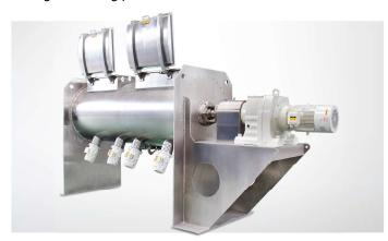
Together with the mixing element, the PerMix Multi-chopper removes lumps in the initial product, chops pasty adhesives and hinders the formation of agglomeration during the moisturizing of powdered substances. The PerMix Multi-chopper is operated independently by its own motor.
